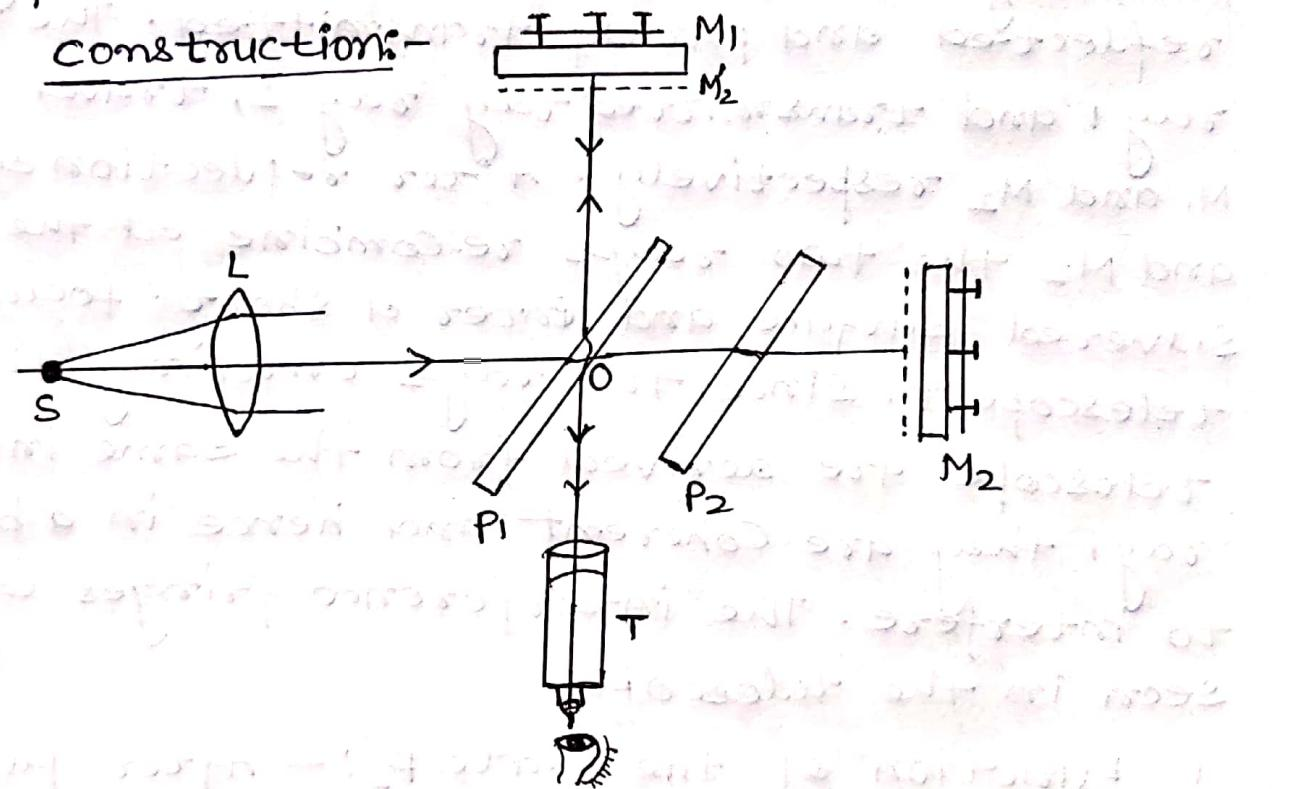
Its main optical parts are two plane mirrors  $M_1$  and  $M_2$  and two similar optically plane, parallel glass plates  $P_1$  and  $P_2$ . The plane mirror  $M_1$  and  $M_2$  are silvered on their front surfaces and are mounted vertically on two arms at right angles to each other. Their planes can be slightly tilted about vertical or horizontal axes by adjusting screws at their backs.
