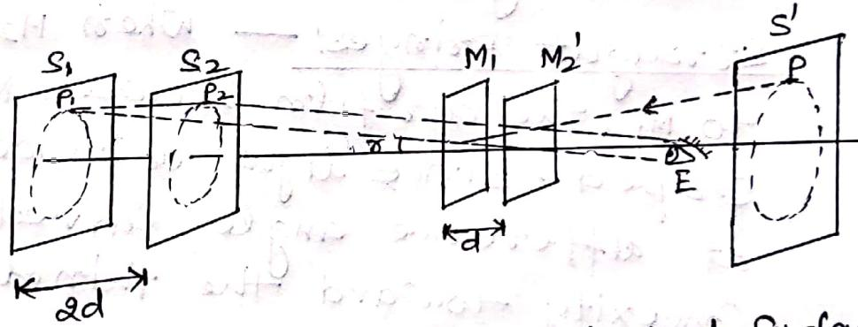
$M_1$  and  $M_2$  are the parallel reflected surfaces. The actual source has been replaced by its virtual image  $S'$  formed by reflection in the partially-silvered surface.  $S'$  from two virtual images  $S_1$  and  $S_2$  in  $M_1$  and  $M'_2$ . The light from a point such as  $P$  on the extended source appear to an eye  $E$  to come from the corresponding coherent points  $p_1$  and  $p_2$  on  $S_1$  and  $S_2$ . If  $d$  is the separation between  $M_1$  and  $M'_2$ , then  $2d$
